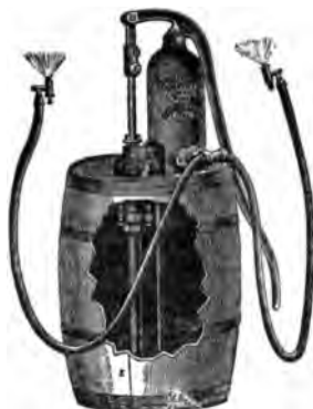
2375. An orchard barrel pump.
